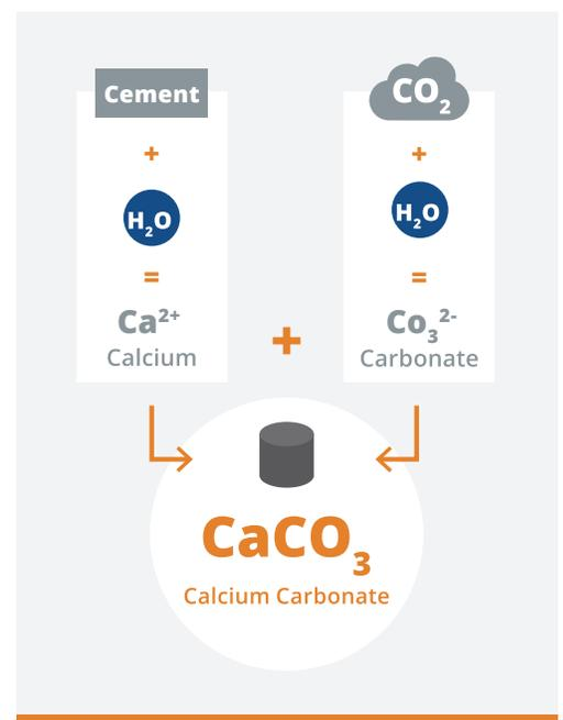
CO<sub>2</sub> mineralization uses waste CO<sub>2</sub> in concrete production. In this process CO<sub>2</sub> is converted to a solid mineral (calcium carbonate), permanently removing these emissions from the atmosphere.
